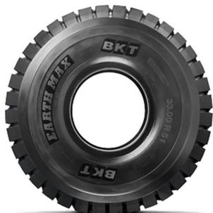
图1 Earthmax SR 46轮胎
